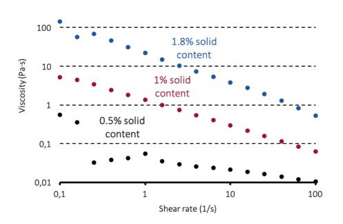
Shear thinning is an important property for achieving great printability at moderate printing pressure. It's also important for the cell's survival upon printing cell-laden bioinks, as the cells would become distorted and broken at too high printing pressure.
