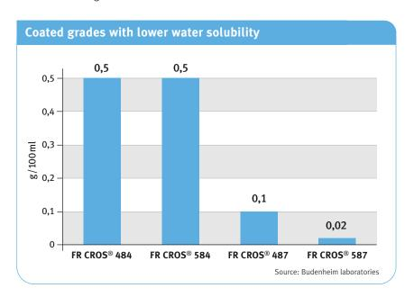
Budenheim developed unique technologies for particle coatings achieving grades of FR CROS® with superior resistance to hydrolysis.
