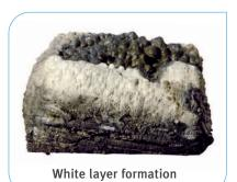
This acid reacts with a carbon source, e.g. based on pentaerythritol, and the coating starts to carbonize without burning. At the same time the **blowing agent** (e.g. melamine) starts to create a carbon foam by releasing gases.
